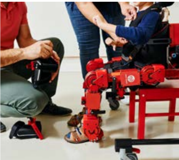
RLS encoders are used in the joints.
