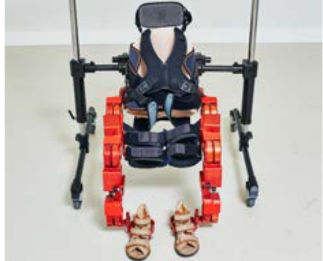
The ATLAS 2030 exoskeleton is designed for children with paraplegia, tetraplegia, spinal muscular atrophy, and congenital muscular dystrophy
