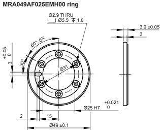
**Dimensions and installation drawings** continued Dimensions and tolerances in mm.
