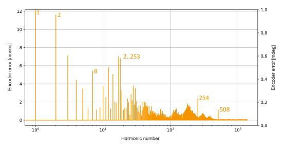
Typical encoder error has some definite higher harmonic components. Example is from the MRA080 + MB080 encoder. Harmonic number:
