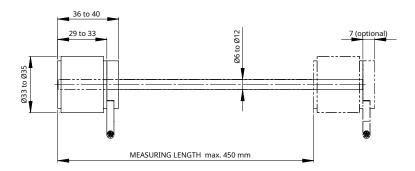
LVDT transducers require coils length greater than the measuring length. Therefore, the sensor head length increases parallel to the measuring length.
