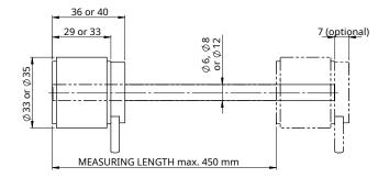
LVDT transducers require coils length greater than the measuring length. Therefore, the sensor head length increases parallel to the measuring length.
