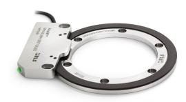
The measuring length of position encoders with a magnetisation period of 1 mm is limited to 230 mm. The maximum rideheight is 0.3 mm. For applications requiring more generous installation tolerances, the maximum distance between the readhead and the scale can be increased, but the measuring length is then reduced to 130 mm.
