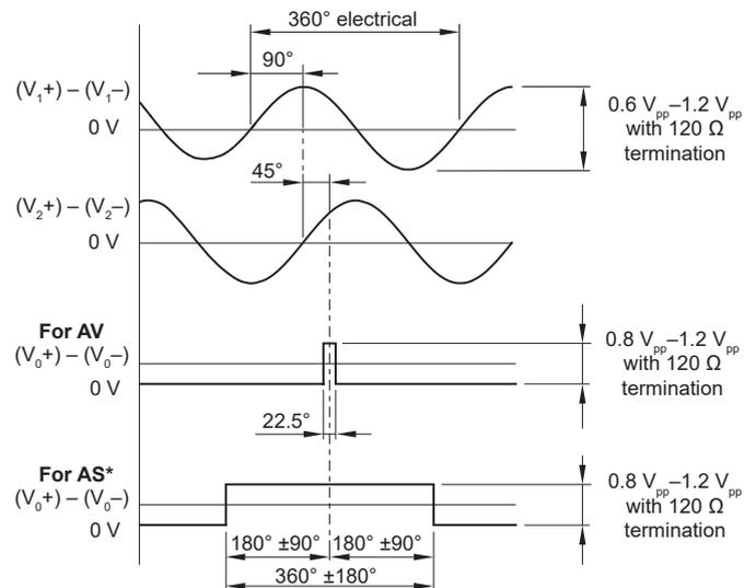
\* AS output type is compatible with controllers (eg. Siemens, Fanuc) with 1 V<sub>pp</sub> encoder inputs.
