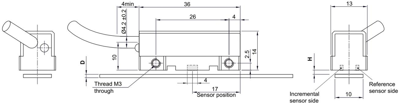
**NOTE:** Ensure recommended M3 readhead fixing screws are tightened to 0.5 Nm to 0.7 Nm.
