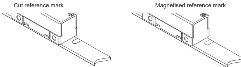
**NOTE:** The shape and position of the cut or magnetised reference are critical so these options are only available as factory order.
