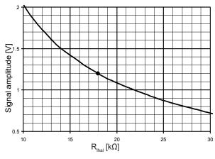
Fig. 31: Signal amplitude as a function of R<sub>Ihal</sub>
