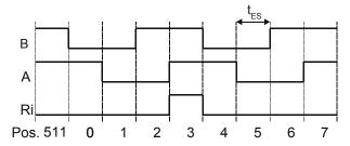
Fig. 6: Timing diagram for incremental output
