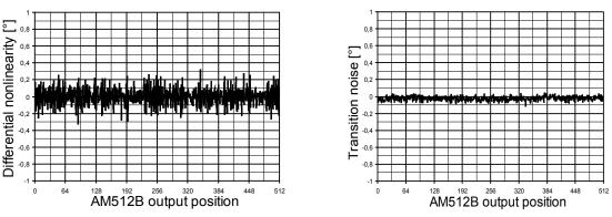
Fig. 17: Typical differential nonlinearity plot
