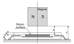
Fig. 21: Cross section of the AM512B with dimensions
