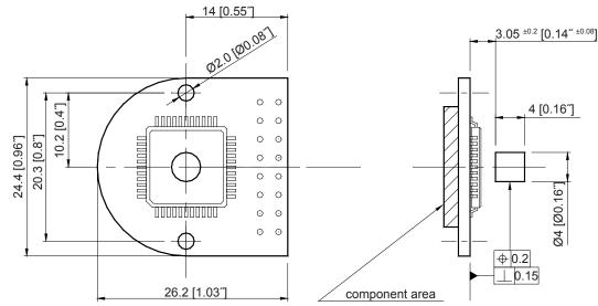
Fig. 41: Dimensional drawing with installation tolerances
