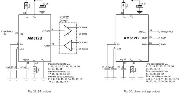
Fig. 30: Linear voltage output
