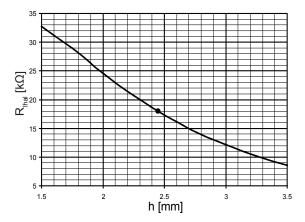
Fig. 34:  $\mathrm{R}_{_{\mathrm{lhal}}}$  to maintain signal amplitude at different h
