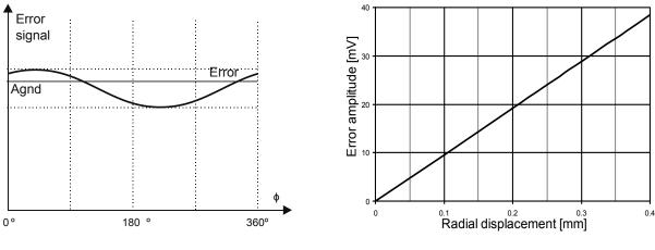
Fig. 25: Error signal shape
