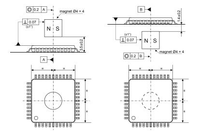
Fig. 22: Mounting instructions for magnet placed above the AM512B and magnet placed beneath the AM512B
