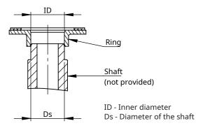
A shoulder on press-fit shaft is highly recommended for parallel alignment.
