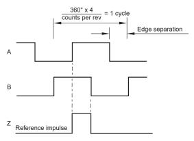
B leads A for clockwise rotation of magnetic actuator.
