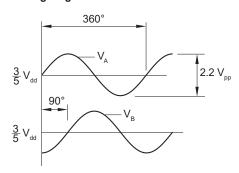
$\rm V_A$  leads  $\rm V_B$  by 90° for clockwise rotation of magnetic actuator.
