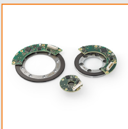
AksIM-2 off-axis absolute magnetic encoder
