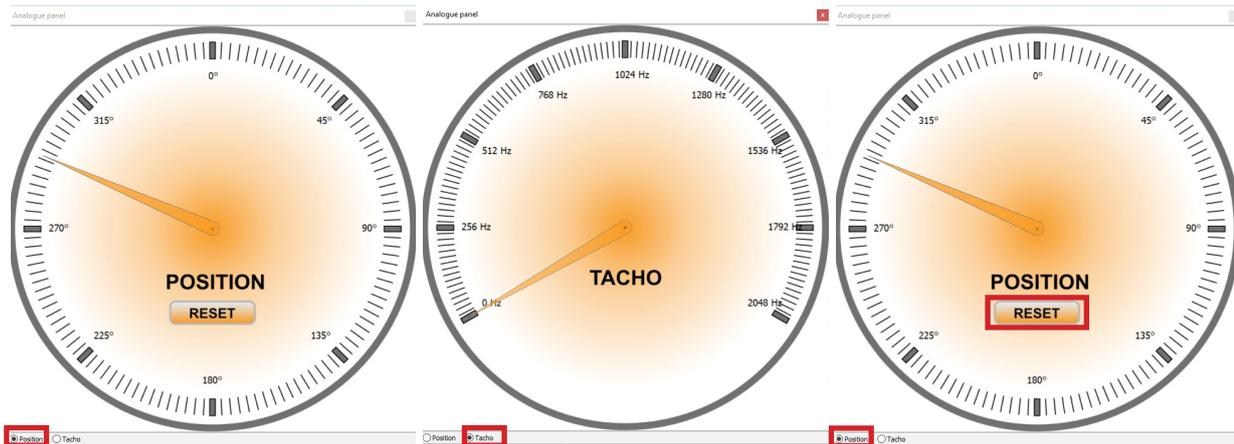
Another display feature is the orange arrow on the very top left hand corner of the main interface. Pressing the arrow will reduce the main interface by hiding the operating board, and moving the digital position display to the top of the interface. Reduced interface can be combined with the analogue display so that the analogue display does not cover the main interface on the screen.
