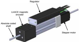
Although combining an encoder with a closed-loop system is no news to the linear actuator world, RLS have taken a step further by developing technology that enables the encoder to read the absolute code written in a solid steel chromecoated shaft. With this innovative feature, to obtain position information by reading directly off the actuator axis, the effect of a system error and environmental conditions on accuracy is minimized.
