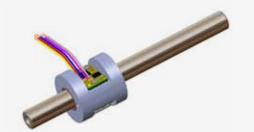
The sensing core of the readhead is a Hall sensor array ASIC. The readhead housing is made of stainless steel with two bronze bearings pressed-in from each side. With the sensor module positioned in between the bearings, the optimal alignment between the sensor module and the shaft is maintained, thus ensuring best performance.
