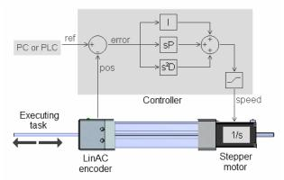
Velocity algorithm controls the position of the piston rod
