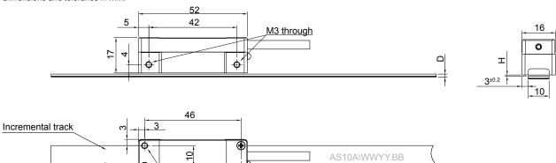
**NOTE:** Orientation of readhead relative to AS10 magnetic tape should be according to drawing. As reference use surface print on AS10 tape or use magnetic viewer (see image below).
