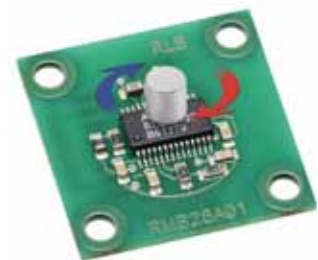
Clockwise (CW) rotation of magnet
