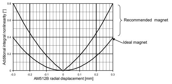
Fig. 24: Additional integral nonlinearity error caused by magnet displacement and quality
