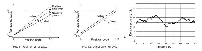
Fig. 13: Typical relative accuracy plot for DAC
