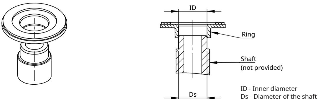
A shoulder on press-fit shaft is highly recommended for parallel alignment.
