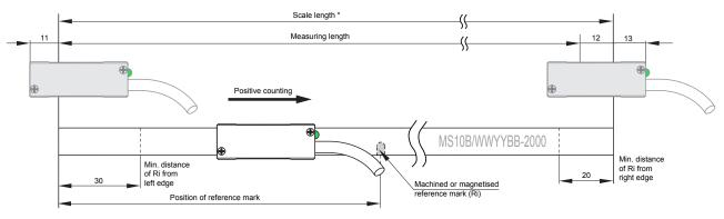
\* Scale length = measuring length + 12 mm
