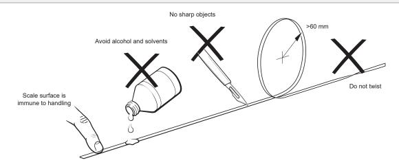
**DO NOT** remove the scale for refitting or use elsewhere once it has been applied to the mounting surface. The scale can be applied once only.
