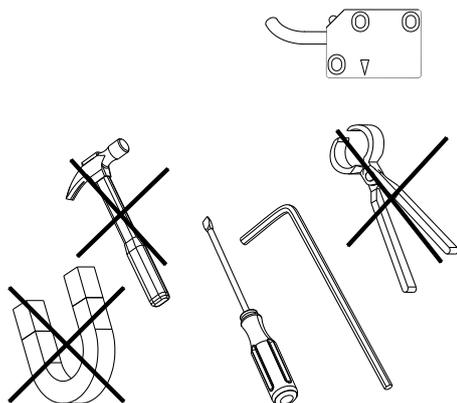
This encoder system is a high performance metrology product and must be handled carefully. The use of industrial tools during installation or exposure to strong magnets such as a magnetic base is not recommended as it carries the risk of damaging parts of the system which as a result might not perform in accordance with specifications.
