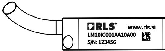
Label on the readhead contains: full PN, 6 digits long serial number and 2D code containing the serial number.
