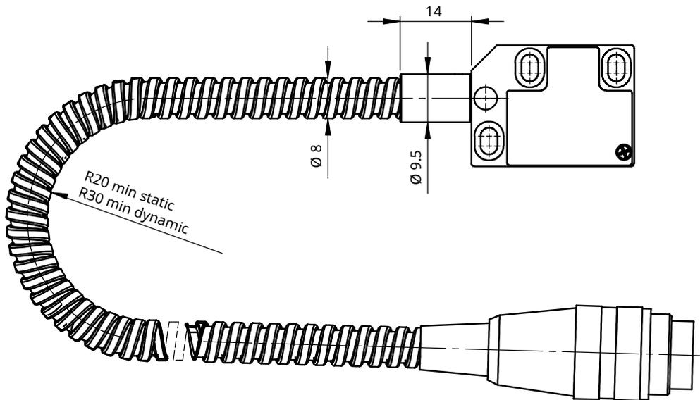
Max. length of cable with flexible stainless-steel conduit is 10 m.
