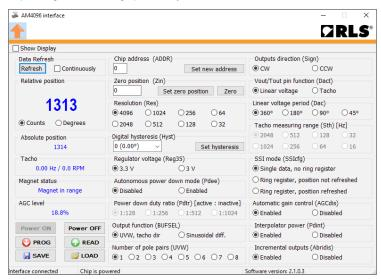
During 'Power on' the interface reads the data stored inside the internal EEPROM of the AM4096 chip and the software interface displays the read information graphically.
