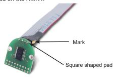
Make sure that the slot on the interfaces is on the same side as the two ridges on the connector.
