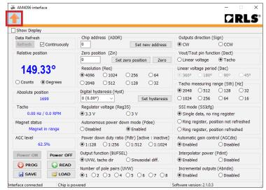
NOTE: All of the changes made will not be programmed to the encoder until the PROG button has been clicked.
