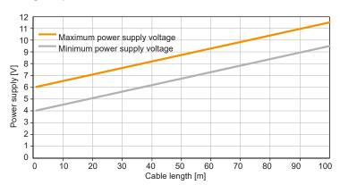
For cables longer than 5 meters input voltage on the cable must be adjusted so the voltage drop is taken into account.
