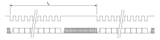
The power supply must be applied at least 10 ms before the clock sequence is being sent to the encoder.
