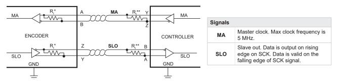
\* The MA and SLO lines are 5 V RS422 compatible differential pairs. The termination resistor on the MA and SLO lines are integrated inside the encoder.
