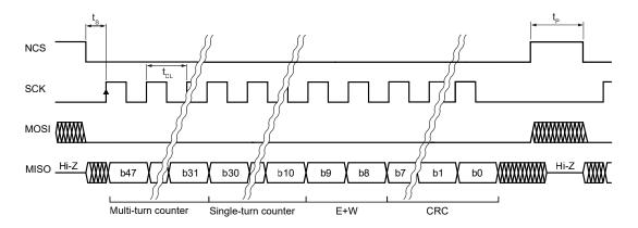
The controller starts the communication by setting the NCS signal low. At the same time the encoder position is latched. A delay of t<sub>s</sub> is required to allow the encoder to prepare the data which is shifted to MISO output on rising edges of clock signal SCK. Encoder Position and General Status (active low) data is transmitted, followed by CRC (inverted) of the entire data packet.
