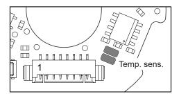
NOTE: Pt1000 sensor can be soldered to the encoder in factory. Contact RLS for availability of this option.
