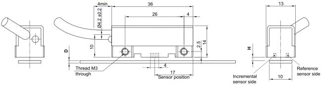
NOTE: Ensure recommended M3 readhead fixing screws are tightened to 0.5 Nm to 0.7 Nm.
