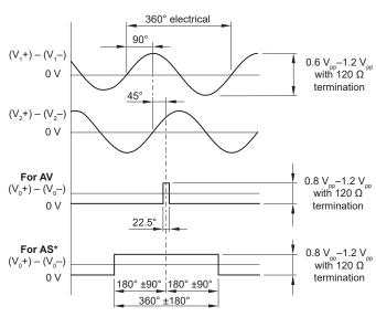
$^{\ast}\,$  AS output type is compatible with controllers (eg. Siemens, Fanuc) with 1  $\rm V_{\rm pp}$  encoder inputs.
