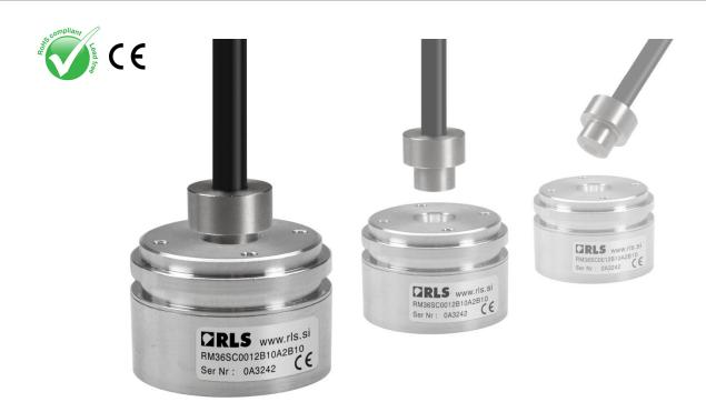
The RM36 is a high-speed magnetic rotary encoder designed for use in harsh industrial environments. The non-contact two-part design removes the need for seals or bearings ensuring long-term reliability and simple installation.
