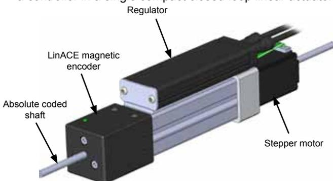
Although combining an encoder with a closed-loop system is no news to the linear actuator world, RLS have taken a step further by developing technology that enables the encoder to read the absolute code written in a solid steel chrome-coated shaft. With this innovative feature, to obtain position information by reading directly off the actuator axis, the effect of a system error and environmental conditions on accuracy is minimized.
