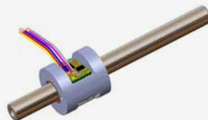
The sensing core of the readhead is a Hall sensor array ASIC. The readhead housing is made of stainless steel with two bronze bearings pressed-in from each side. With the sensor module positioned in between the bearings, the optimal alignment between the sensor module and the shaft is maintained, thus ensuring best performance.
