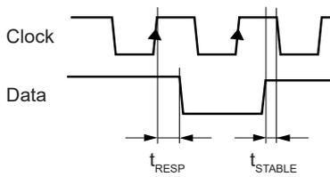
The readhead needs 170 ns to respond to incoming clocks ( $t_{RESP}$ ). Change on Data signal is delayed for 170 ns after the rising edge on Clock line. Additional delay is caused by the time the signal needs to propagate through cable to the readhead and back ( $t_{PROP}$ ). This delay is typically 14 ns per 1 meter of cable. Data signal must be stable for at least 10 % of the clock period length before the value is latched.
