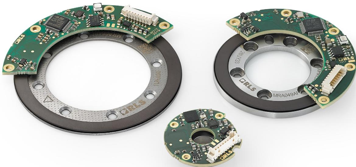
**AksIM-2 is a non-contact, high performance off-axis absolute rotary encoder designed for integration into applications with limited space. A hollow ring, true absolute functionality and high-speed operation make this encoder suitable for many applications.**
