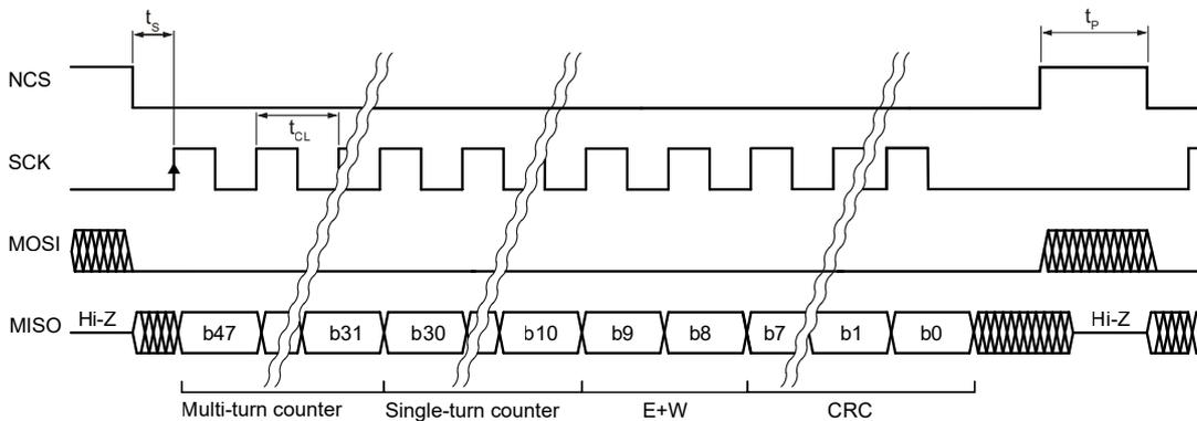
The controller starts the communication by setting the NCS signal low. At the same time the encoder position is latched. A delay of  $t_s$  is required to allow the encoder to prepare the data which is shifted to MISO output on rising edges of clock signal SCK. Encoder Position and General Status (active low) data is transmitted, followed by CRC (inverted) of the entire data packet.
