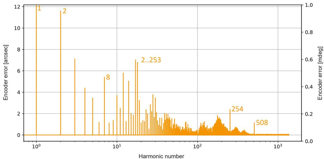
Typical encoder error has some definite higher harmonic components. Example is from the MRA080 + MB080 encoder. Other encoder sizes have slightly different spectrum.
