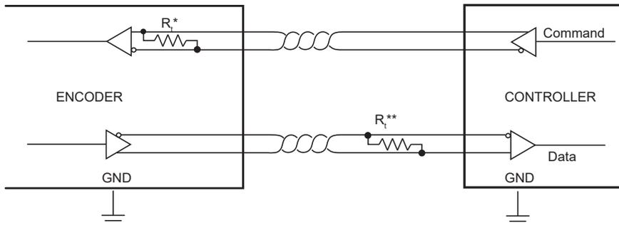
\* The Command and Data signals are 5 V RS422 compatible differential pairs with RC termination inside the readhead.
