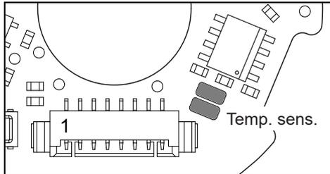
NOTE: Pt1000 sensor can be soldered to the encoder in factory. [Contact RLS](#) for availability of this option.
