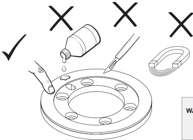
**WARNING:** Magnetic rings should not be exposed to magnetic field densities higher than 50 mT on its surface. Magnetic fields higher than 50 mT can damage the ring.
