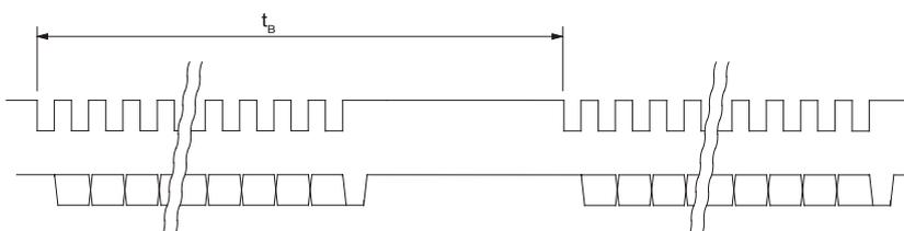
The power supply must be applied at least 100 ms before the clock sequence is being sent to the encoder.
