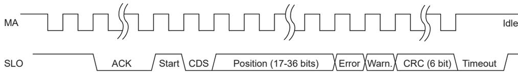
MA is idle high. Communication is initiated with first falling edge.
