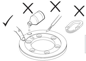
WARNING: Magnetic rings should not be exposed to magnetic field densities higher than 50 mT on its surface. Magnetic fields higher than 50 mT can damage the ring.
