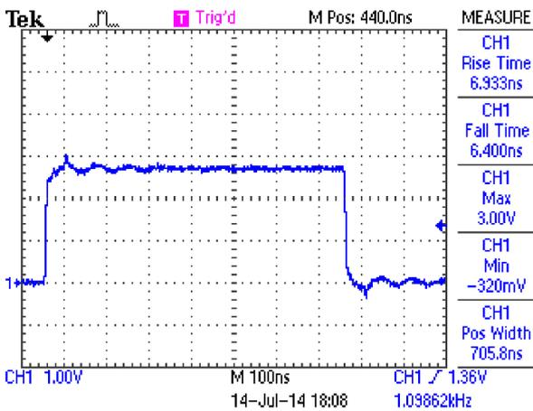
Termination reduces ringing and overshoots to nearly zero but signal drop is noticeable. Voltage is 2.8 V.
