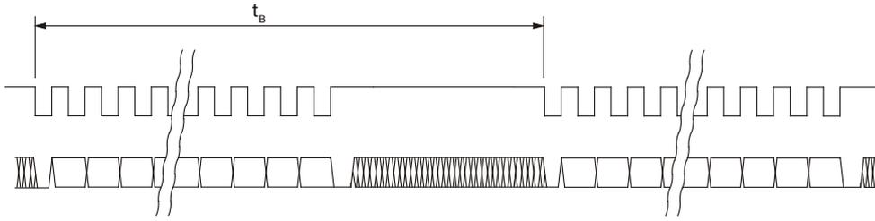
The power supply must be applied at least 10 ms before the clock sequence is being sent to the encoder.
