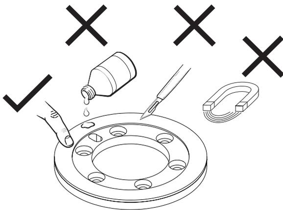
**HANDLE WITH CARE.** This encoder system is a high performance metrology product and should be treated with the same care as any other precision instrument. Use of heavy duty industrial tools or exposure to strong magnets, such as a magnetic base, is unacceptable and risks of irreparable damage to the product.
