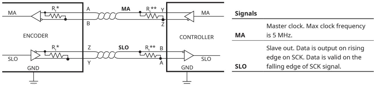
\* The MA and SLO lines are 5 V RS422 compatible differential pairs. The termination resistor on the MA and SLO lines are integrated inside the encoder.
