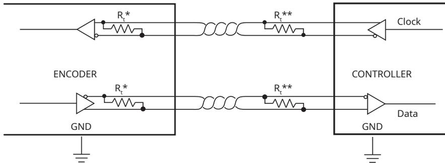
\* The Clock and Data signals are 5 V RS422 compatible differential pairs with RC termination inside the readhead.
