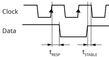
The readhead needs 170 ns to respond to incoming clocks ( $t_{RESP}$ ). Change on Data signal is delayed for 170 ns after the rising edge on Clock line. Additional delay is caused by the time the signal needs to propagate through cable to the readhead and back ( $t_{PROP}$ ). This delay is typically 14 ns per 1 meter of cable. Total cable length must be taken into account, from the encoder to the receiver.
