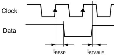
The readhead needs 170 ns to respond to incoming clocks ( $t_{RESP}$ ). Change on Data signal is delayed for 170 ns after the rising edge on Clock line. Additional delay is caused by the time the signal needs to propagate through cable to the readhead and back ( $t_{PROP}$ ). This delay is typically 14 ns per 1 meter of cable. Data signal must be stable for at least 10 % of the clock period length before the value is latched.
