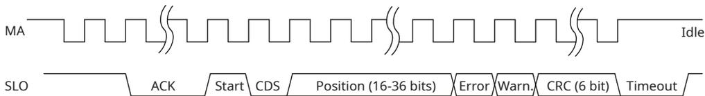
MA is idle high. Communication is initiated with first falling edge.
