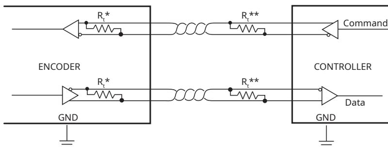
\* The Command and Data signals are 5 V RS422 compatible differential pairs with RC termination inside the readhead.
