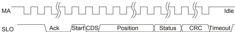
MA line is idle high. Communication is initiated with first falling edge. The encoder responds by setting SLO low on the second rising edge on MA. When the encoder is ready for the next request cycle it indicates this to the master by setting SLO high. The absolute position and CRC data is in binary format and sent MSB first.
