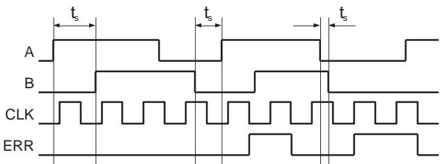
Error is detected when less than two fronts of **CLK** signal are inside **A**, **B** signals separation time ( $t_s$ ). **ERR** signal appears at second next **CLK** front and lasts for one **CLK** period.
