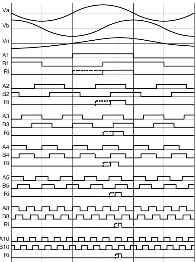
\* ----- Msel use to select index pulse duration (equal to A track – 180 deg or A/B overlap – 90 deg)
