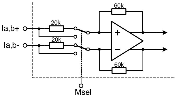
The default gain is 3 for differential **Voltage inputs** – default setting.
