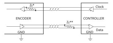
\* The Clock and Data signals are 5 V RS422 compatible differential pairs with RC termination inside the readhead.
