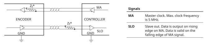
\* The MA and SLO lines are 5 V RS422-compatible differential pairs. The termination resistor on the MA line is integrated in the encoder.
