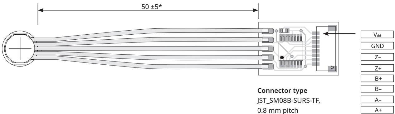
\* Differential output available with soldered LDB01 and added strain relief on 50 mm distance from the RM08.
