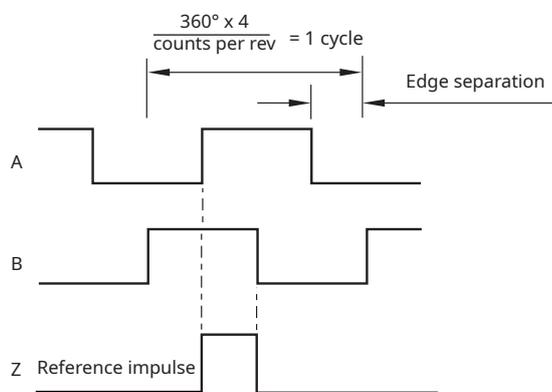
B leads A for clockwise rotation of magnetic actuator.
