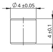
**Fixing:** Adhesive (recommended – LOCTITE 648 or 2701)
