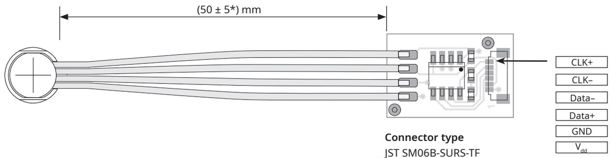
\* Differential output available with soldered LDB02 and added strain relief on 50 mm distance from the RM08.
