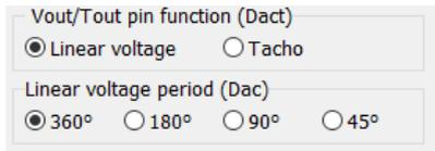
If 'Vout' is selected, the period of the linear voltage output can be selected. See page 14 of the AM4096D01 datasheet for a detailed description of the Linear voltage output.
