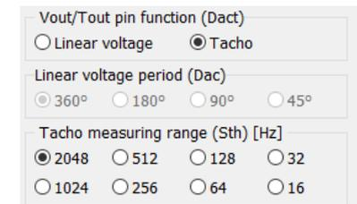
If 'Tacho' is selected, the measuring range can be selected (in Hz). See page 13 of the AM4096D01 datasheet for a detailed description of the Tacho output.
