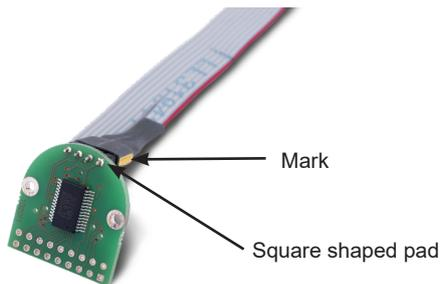
Make sure that the slot on the interfaces is on the same side as the two ridges on the connector.
