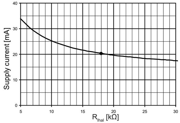
Fig. 36: Supply current as a function of R<sub>thermal</sub>
