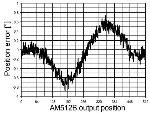
Fig. 16: Typical integral nonlinearity plot if the magnet is on the limit of alignment tolerances
