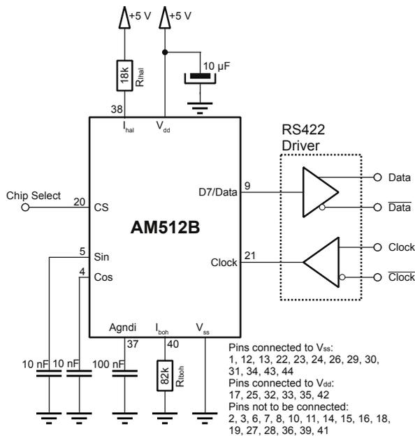
Fig. 29: SSI output
