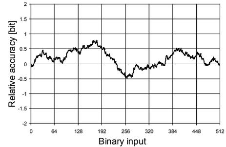
Fig. 13: Typical relative accuracy plot for DAC
