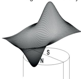
Fig. 19: Distribution of the perpendicular component of  $B$
