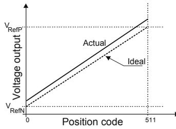
Fig. 12: Offset error for DAC
