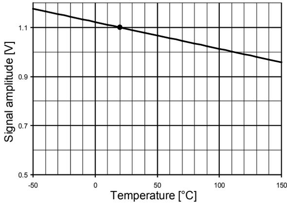
Fig. 35: Signal amplitude as a function of temperature
