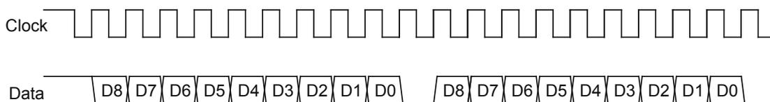
Fig. 5: SSI multi-read of the same position data
