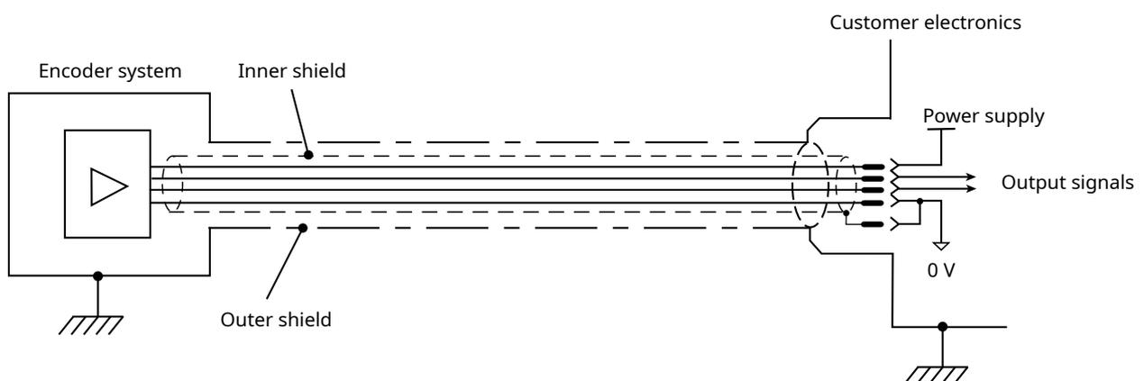
Housing of the encoder is galvanically connected with the housing of the connector via the cable outer shield. The encoder system must be correctly integrated to achieve EMC compliance. In particular, attention to shielding arrangements is essential.
