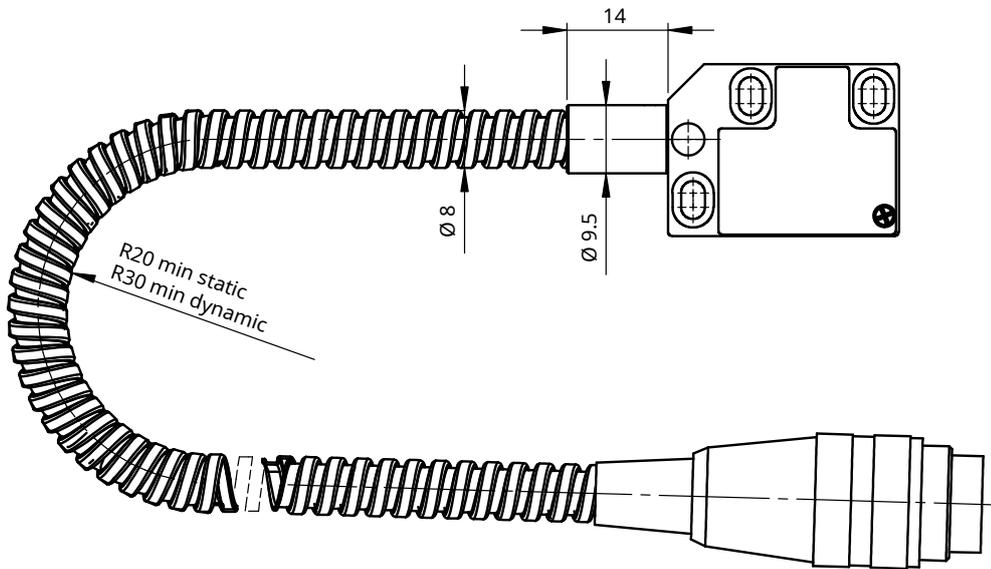
Max. length of cable with flexible stainless-steel conduit tube is 10 m.
