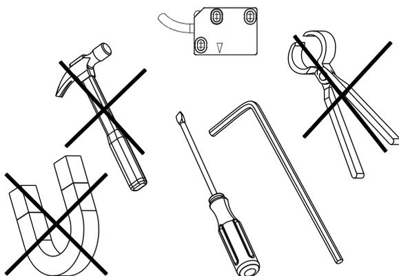
This encoder system is a high performance metrology product and must be handled carefully. The use of industrial tools during installation or exposure to strong magnets such as a magnetic base is not recommended as it carries the risk of damaging parts of the system which as a result might not perform in accordance with specifications.
