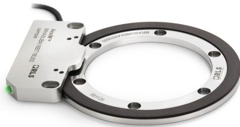
The measuring length of position encoders with a magnetisation period of 1 mm is limited to 230 mm. The maximum rideheight is 0.3 mm. For applications requiring more generous installation tolerances, the maximum distance between the readhead and the scale can be increased, but the measuring length is then reduced to 130 mm.
