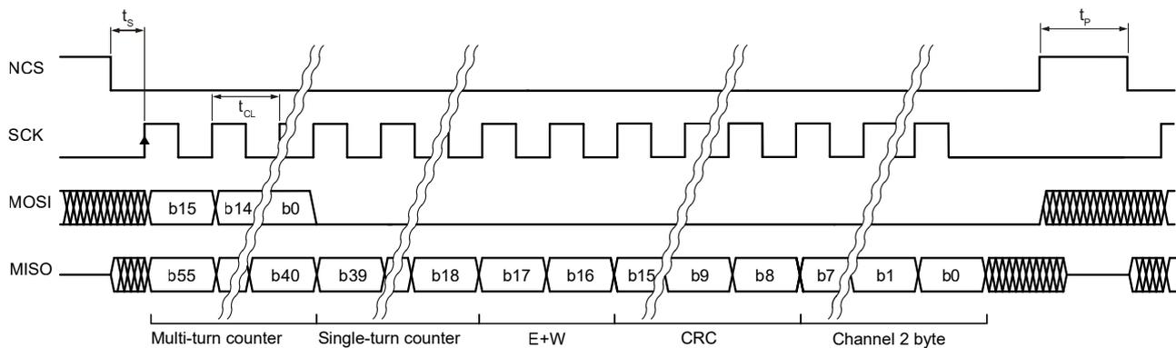
Controller starts the communication by setting the NCS signal low. At the same time the encoder position is latched. A delay of  $t_s$  is required to allow the encoder to prepare the data which is then shifted to MISO output on rising edges of clock signal SCK. Encoder Position and General Status (active low) data is transmitted, followed by CRC (inverted) of the first part of the data packet. Last byte (after CRC) is used by the EncoLink library to transfer data from protocol layers 2 and 3.
