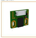
RLC2IC with through-hole pads
