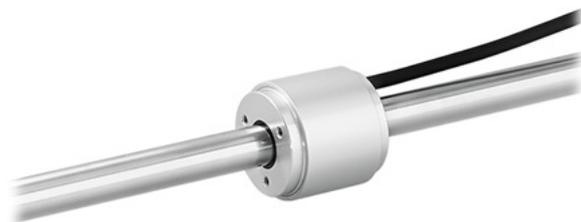
Although these encoders operate on the principle of magnetic field sensing, they have excellent resistance to stray magnetic fields. The hard-chrome plated coded shaft is not magnetised and cannot be damaged by stray magnetic fields.
