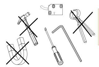
This encoder system is a high performance metrology product and must be handled carefully. The use of industrial tools during installation or exposure to strong magnets such as a magnetic base is not recommended as it carries the risk of damaging parts of the system which as a result might not perform in accordance with specifications.
