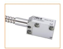
LM15 with cable with flexible stainless-steel conduit which is excellent for harsh environments. It comes with standard LM15 outputs.
