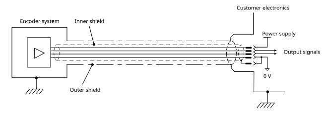
Housing of the encoder is galvanically connected with the housing of the connector via the cable outer shield. The encoder system must be correctly integrated to achieve EMC compliance. In particular, attention to shielding arrangements is essential.
