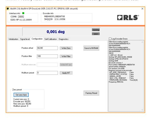
5. To ensure optimal performance of the encoder, it is possible to perform a self-calibration in the "Self-Calibration" section. For details refer to the encoder's data sheet MBD08 at **RLS Media center.**
