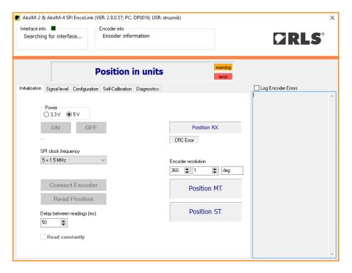
2. When the interface is found, first select power type of your encoder and then press "ON" (your encoder will turn on). Then connect the encoder and press "Read Position" (if you want to have a constant information about the position check the box "Read constantly").
