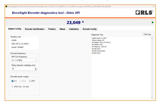
2. The "Encoder Identification" section provides information about the connected encoder. If an older version of the Orbis encoder is used, only the serial number and multiturn information is displayed and the magnet size must be entered manually. If a newer version of the encoder is used, the part number and firmware version are also displayed and the magnet size is set automatically.
