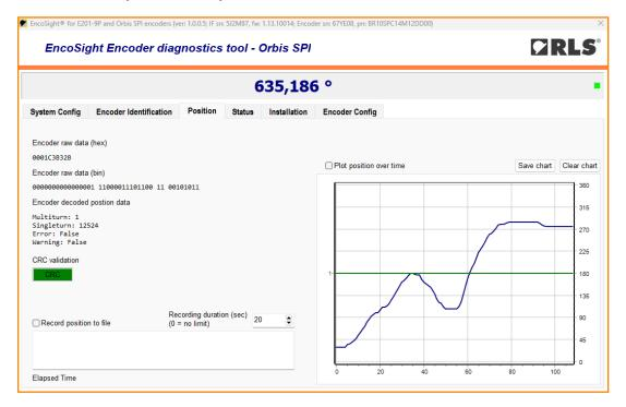
4. The detailed status of the encoder, including the status bits and their descriptions, can be found in the "Status" section. This section also contains information about the temperature, speed and timestamp of the encoder.
