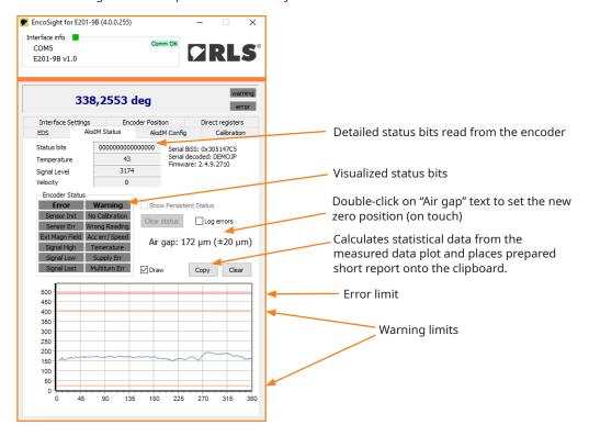
7. To ensure optimal performance of the encoder, it is possible to perform a self-calibration in the "Calibration" menu. For more information about the self-calibration function, refer to the data sheet of the connected encoder.
