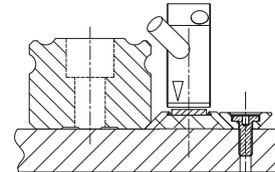
Reference surface available for alignment of track section.
