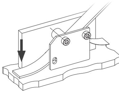
To prevent the scale sticking to the mounting surface during this operation it may be necessary to re-apply approximately 20 mm of backing paper to the end of the scale before inserting through applicator tool.
