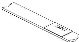
Do not remove the scale for refitting or use elsewhere once it has been applied to the mounting surface. The scale can be applied only once.
